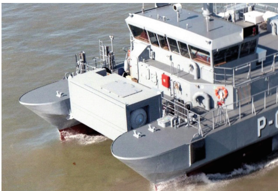
Fig. 4. Small Waterplane Area Twin Hull with mission's module [8].
