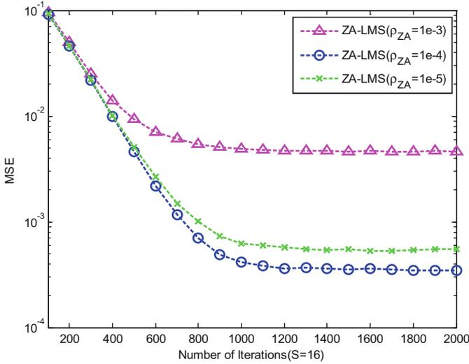
Fig. 10. ZA-LMS simulation with different  $\rho_{ZA}$  values.
