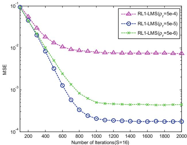
Fig. 12. RL1-LMS simulation with different  $\rho_r$  values.
