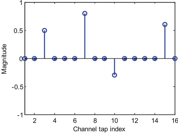
**Fig. 1.** Example of typical sparse channel model.
