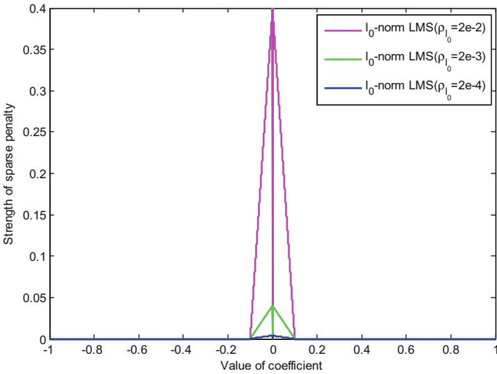
**Fig. 8.** Sparse constraints to channel vector  $\mathbf{w}$  of  $\ell_0$ -norm LMS algorithm with different  $\rho_r$  values ( $\beta = 10$ ).
