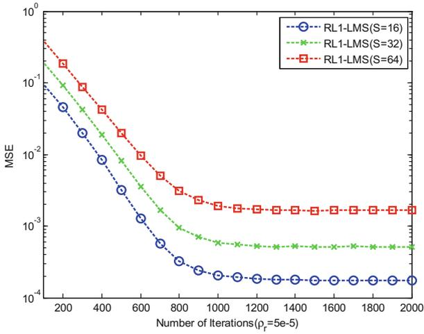
Fig. 17. Simulation of RL1-LMS algorithm with different S.
