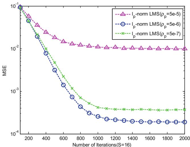
Fig. 13.  $l_p$ -norm LMS simulation with different  $\rho_p$  values.
