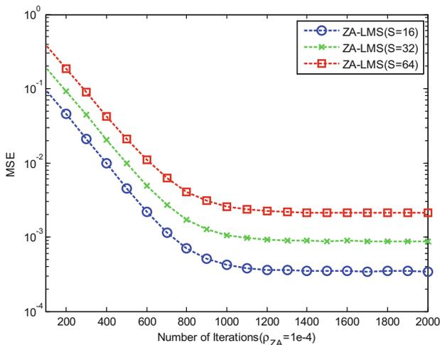
Fig. 15. Simulation of ZA-LMS algorithm with different S.
