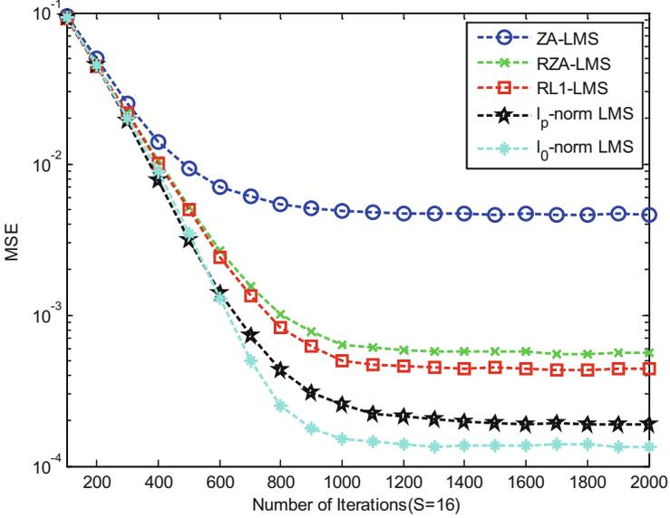
Fig. 9. Comparisons between different sparse LMS algorithms.
