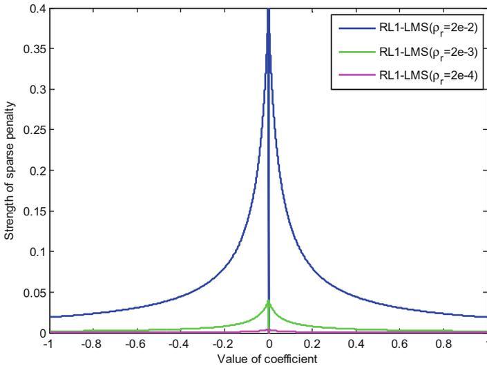
**Fig. 6.** Sparse constraints to channel vector  $\mathbf{w}$  of RL1-LMS algorithm with different  $\rho_r$  values ( $\epsilon_r = 5 \times 10^{-2}$ ).
