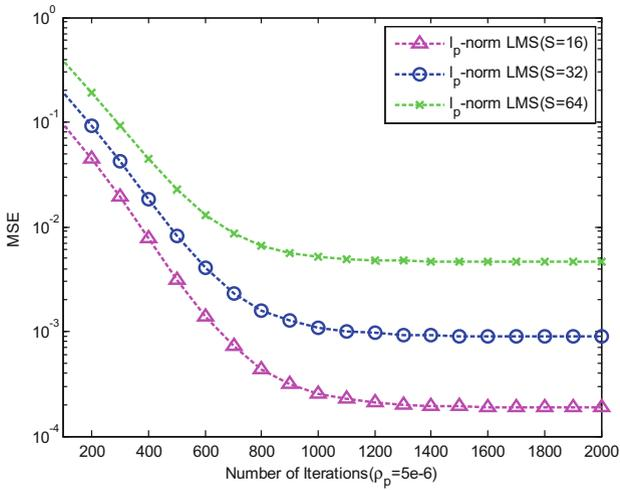
Fig. 18. Simulation of  $l_p$ -norm LMS with different S.
