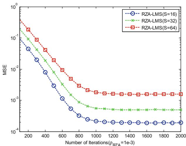
Fig. 16. Simulation of RZA-LMS algorithm with different S.
