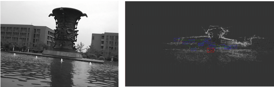
Fig. 7. The left picture shows the source picture. And the right one is the result of SIFT-SLAM algorithm.
