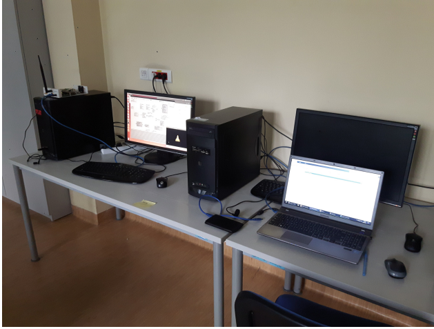
Fig. 2. Photograph of the first white-space transceiver (left side computer with USRP board put on it) and REM database (right computer connected with Internet via Ethernet cable); the left-side computer communicates with database using WLAN-dongles stick into it
