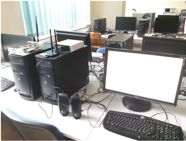
Fig. 3. Photograph of the second white-space transceiver (the one with USRP board laying on it); the computer communicates with database using WLAN-dongles
