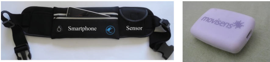
Fig. 2. Waistbelt and movisens Move II accelerometer.
