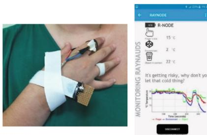
**Fig. 4.** Working prototype and its application interface.
