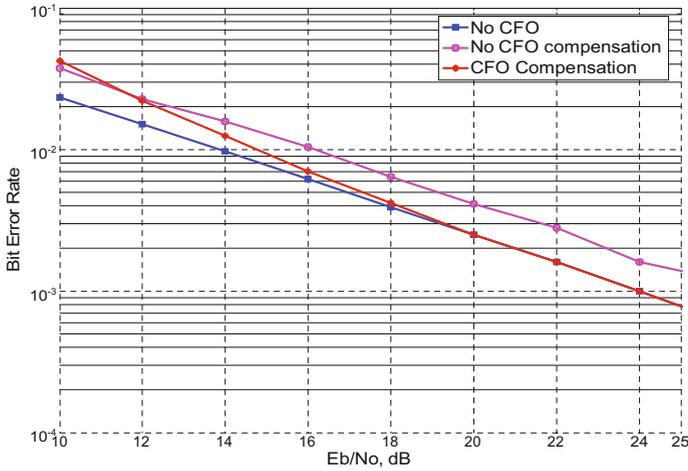
Fig. 6. BER with and without CFO compensation
