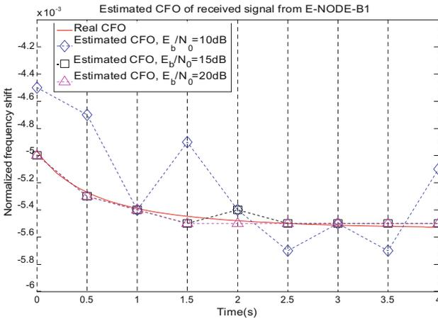
**Fig. 3.** The estimated CFO and the actual CFO at E-NODE-B1
