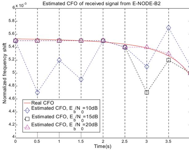
Fig. 4. The estimated CFO and the actual CFO at E-NODE-B2
