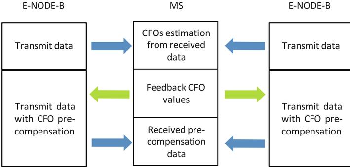
**Fig. 2.** Scheme for pre-compensation CFOs communication
