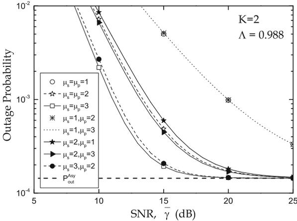
**Fig. 4.** Outage probability for various Nakagami- $m$  fading severity with  $\Xi = 1.44E-4$ .
