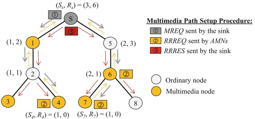
Fig. 4. An example of path setup procedure
