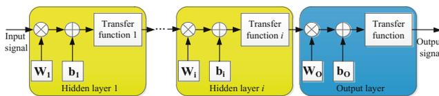
Fig. 4. Structure of feed forward network (FFN)
