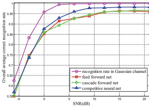
Fig. 8. Overall average correct recognition rate vs. SNR
