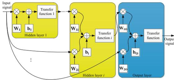
Fig. 5. Structure of cascade forward network (CFN)
