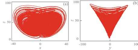
**Fig. 5.** Chaotic attractor of Bao hyperchaotic system: (a)  $x$ - $z$  plane (b)  $y$ - $z$  plane
