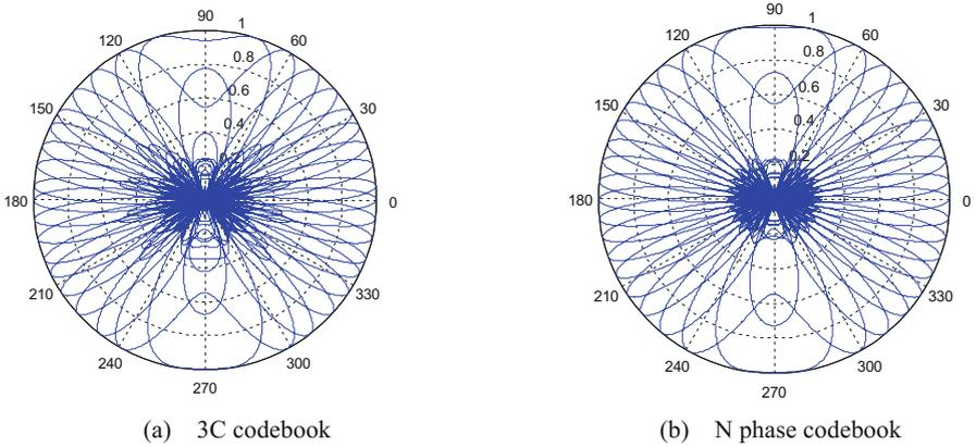
**Fig. 4.** Normalized polar coordinate beam pattern
