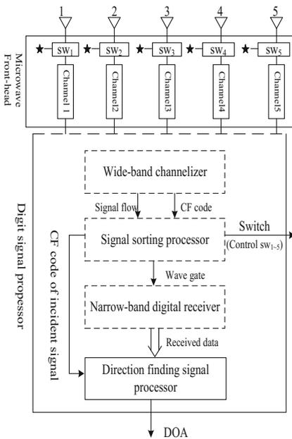
Fig. 3. Block diagram of the DF system
