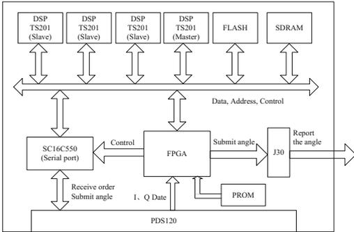
**Fig. 5.** Diagram of the DF signal processor
