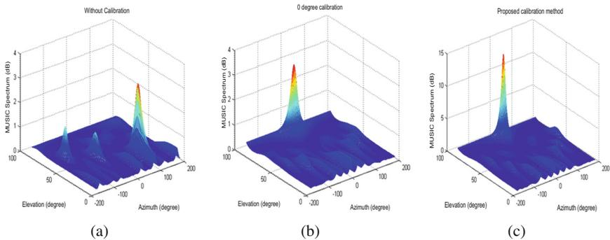
**Fig. 7.** MUSIC spectrum of DOA estimation under the condition of (a) without calibration (b)  $0^\circ$  calibration method (c) proposed calibration method
