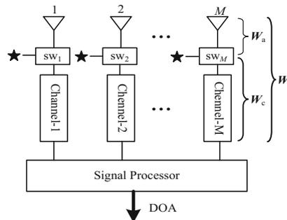
Fig. 2. Diagram of data receiving in DF system.
