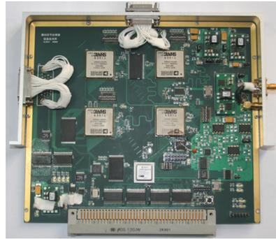
**Fig. 6.** Appearance of the DF signal processor
