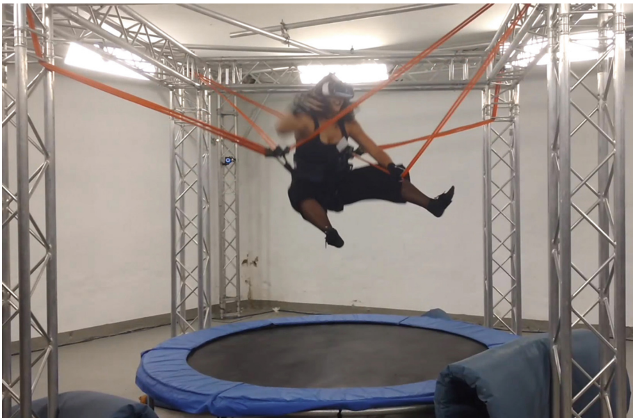
Fig. 2. Evaluation setup with elastic ropes. User in a belt jumping in a seating position to avoid the next incoming space ship obstacle.
