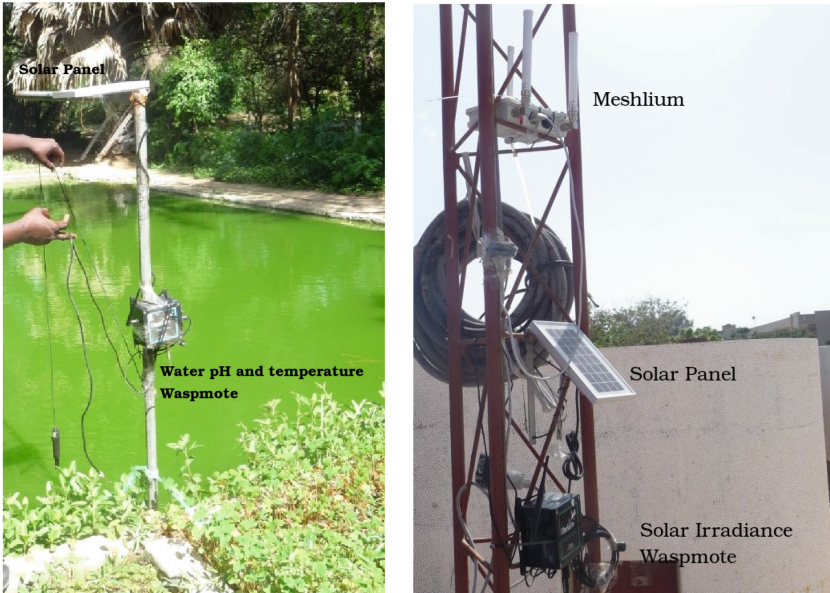
(a) Water pH and temperature measurement kit (b) Meshlium gateway and solar irradiance measurement kit
