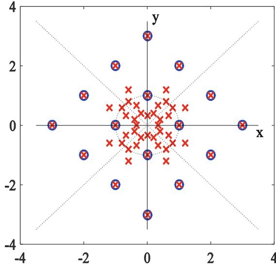
**Fig. 1.** 16QAM constellation (“○”) and  $\frac{g_u}{g_v}$  results (“×”)
