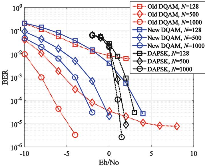
**Fig. 2.** BER performance of differential 16QAM and 16DAPSK
