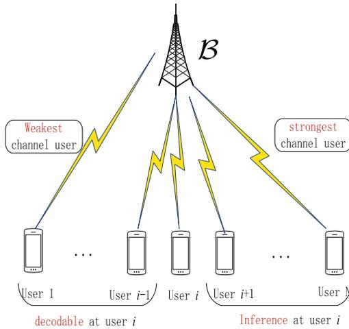
**Fig. 1.** Multiuser downlink system topology.
