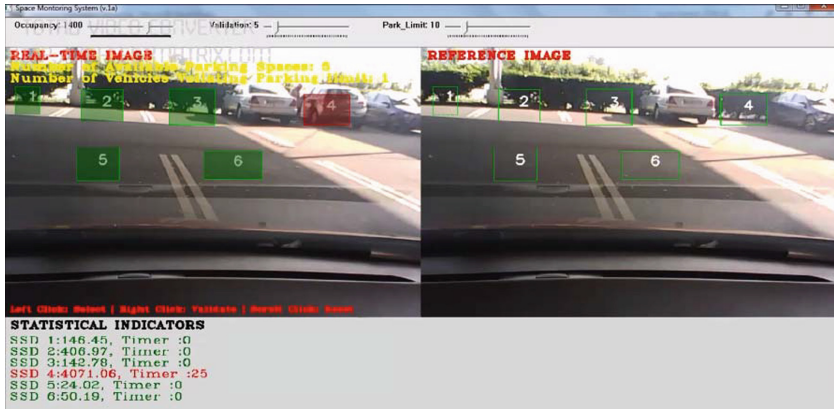
Fig. 3. System developed for the automatic detection of available parking slots in real-time [7, 8, 10]. Slots colorized in green and red represents detected vacant and occupied slots, respectively (color figure online).
