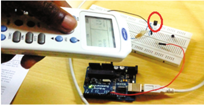
Fig. 2. Signal code capture from a legacy remote control via an infrared receiver.
