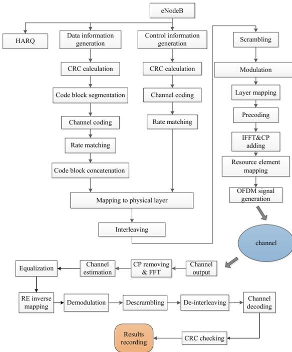
**Fig. 5.** The flow chart of LTE downlink process.
