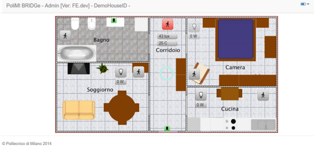
Fig. 1. Live perspective of the house status. In this visualization the person is localized in the corridor (cyan ring), and the corresponding movement sensor (in red) is triggered. (Color figure online)
