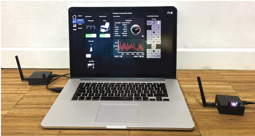
Fig. 4. The iHouse smart home server application running on a PC connected to the receiver module over USB, Line in and Line out. A microphone module is shown on the right side. On the left side of the app, the room of interest can be selected. In the center, all available devices in this selected room are shown and can be controlled.
