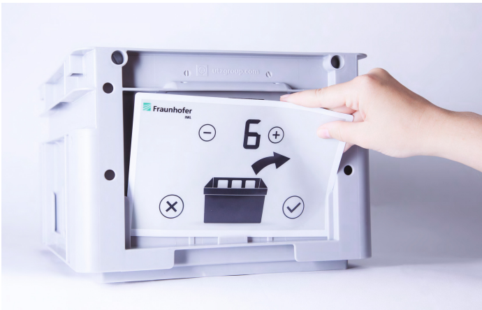
Fig. 7. A P-ink system easily mounted on a standard size bin courtesy Fraunhofer IML, Dortmund
