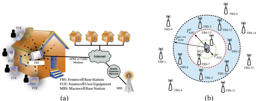
**Fig. 1.** (a) Illustration of femtocell [5] and (b) applying the MDA of the handoff mechanism. (Color figure online)
