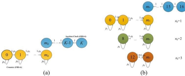
**Fig. 2.** The counter and auction clock of candidate FBS- $k$  in the (a) SEP and (b) fast SEP.
