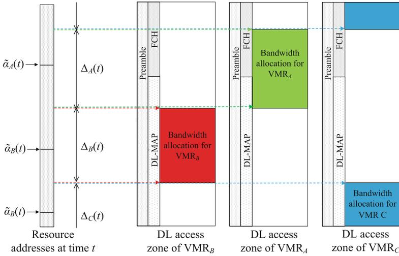
**Fig. 3.** Example of resource allocation among VMR<sub>A</sub>, VMR<sub>B</sub> and VMR<sub>C</sub>
