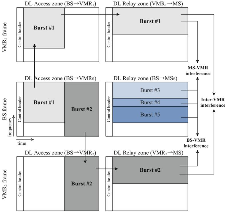
**Fig. 2.** Relay frame structure in IEEE 802.16j
