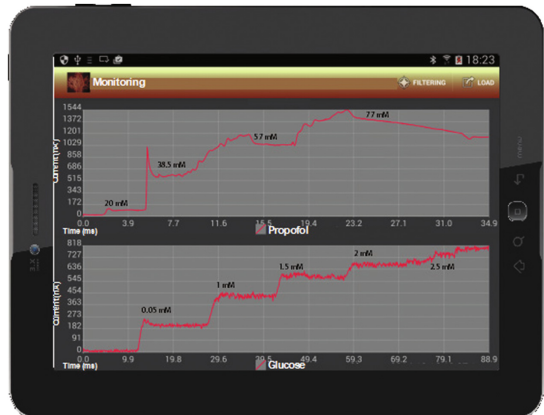
Fig. 2. Measure values displayed on bedside Client tablet. Monitored parameters are: endogenous glucose and exogenous propofol anesthetic.
