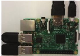
Fig. 5. Fog computing unit, with developed bot is realized on Raspberry Pi 3.
