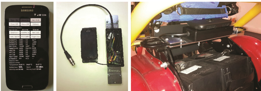
Fig. 2. The Galaxy S4 smartphone running the app (left), a view of the devices placed in the plastic box and rugged enclosure (center). Final setup in the back side of the wheelchair (right) with the custom metal plate.
