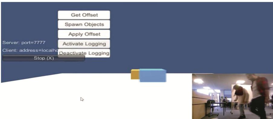
**Fig. 1.** An example snapshot from the video where the cameras were placed at the edges of the scene view. A single camera would provide an occluded image, but two cameras keep track of two people, represented by the blue and yellow cuboids. (Color figure online)
