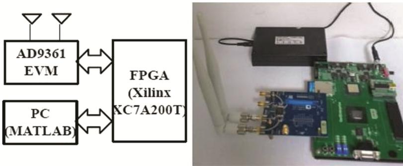
**Fig. 6.** Software defined radio platform with AD9361 EVM and Xilinx/SMIMS AC701 evaluation board
