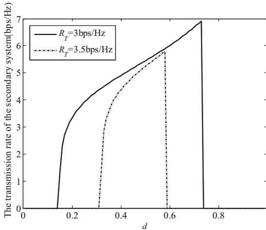
**Fig. 2.** The rate of secondary system with various  $R_T$  versus different position of ST
