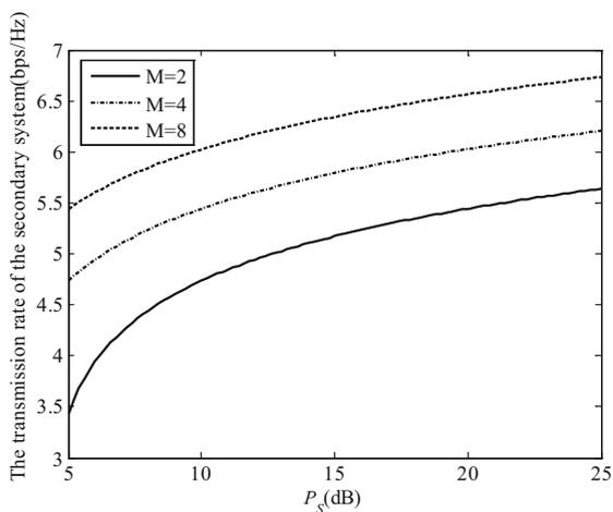
**Fig. 4.** The rate of secondary system with various  $M$  versus different  $P_S$
