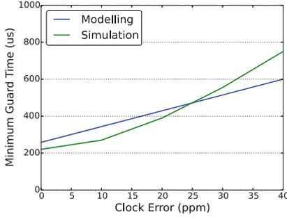
(a) Minimum guard time for operation without packet loss.
