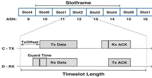
**Fig. 2.** A typical TSCH timeslot template for a transmitter (top) and receiver node (bottom): node C, transmits its data packet after **TxOffset**, while the receiver D, uses a **Guard Time** to avoid missing the incoming packet by turning its radio on slightly before the packet arrival.
