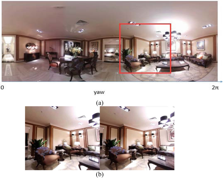
Fig. 4. Illustration of adaptive playback of the Pseudo-3D panoramic video: (a) a frame in panoramic video (b) when yaw = 1.4\pi , the scene mix True-3D and Pseudo-3D method to present video content to the viewers adaptively.
