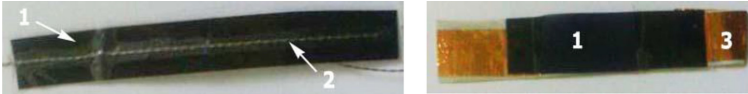
Fig. 2. Velostat based sensor prototypes: Velostat track (1) with steel thread (2) (left) and Velostat track (1) with copper ribbon (3) (right).
