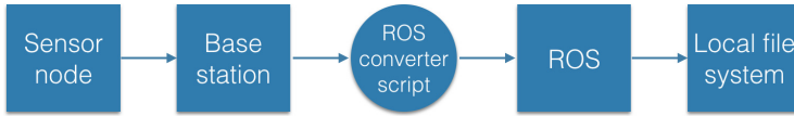
Fig. 2. Data flow diagram of patient data within the boundary of the apartment
