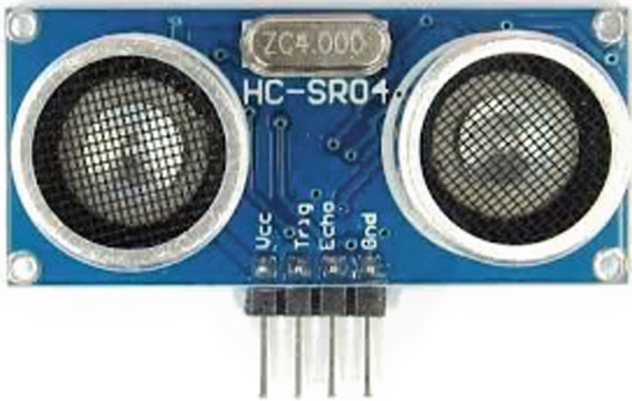
Fig. 2. An HC-SR04 type ultrasonic sensor
