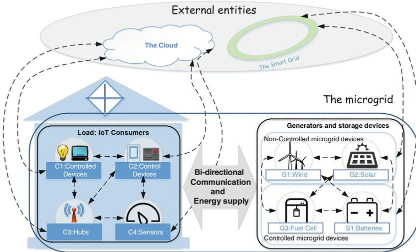
Fig. 2. IoT-microgrid architecture.
