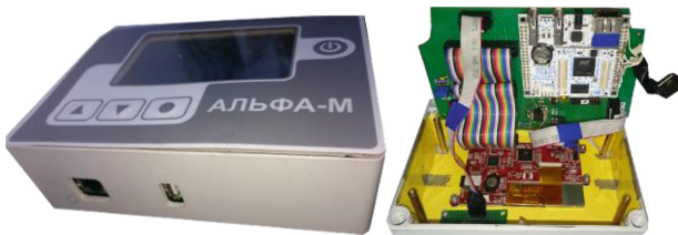
Fig. 3. External and internal views of the control device.
