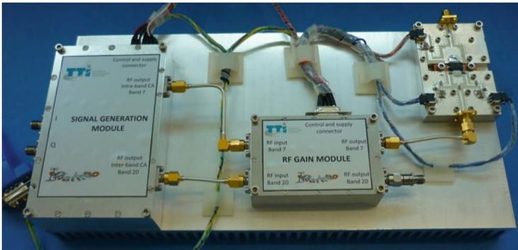
**Fig. 8.** Picture of the reconfigurable RF front-end prototype.
