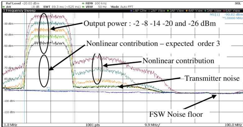
Fig. 7. Transmitted spectrum for different output powers
