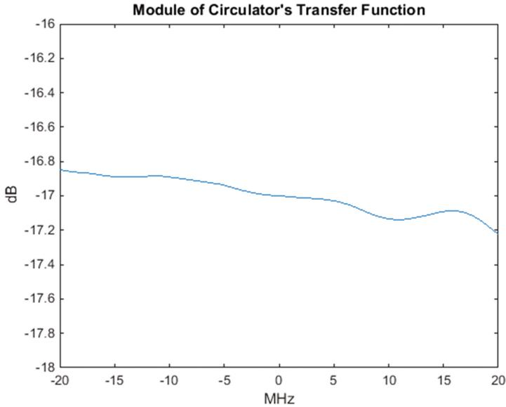
**Fig. 2.** Equivalent baseband circulator and antenna frequency response
