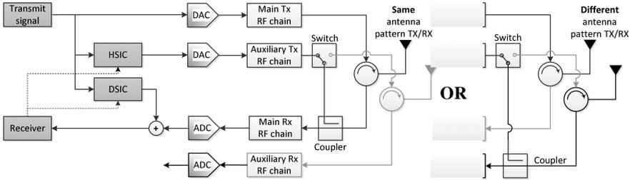
Fig. 1. In-band Full-duplex transceiver using MIMO architecture
