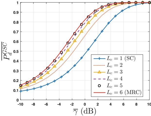
Fig. 4. Variation of detection probability versus  $\bar{\gamma}$  with  $N = 1$ ,  $L = 6$  and  $P_{fa} = 0.05$ .
