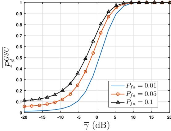
Fig. 3. Variation of detection probability versus  $\bar{\gamma}$  with  $N = 1$ ,  $L = 4$  and  $L_c = 3$ .
