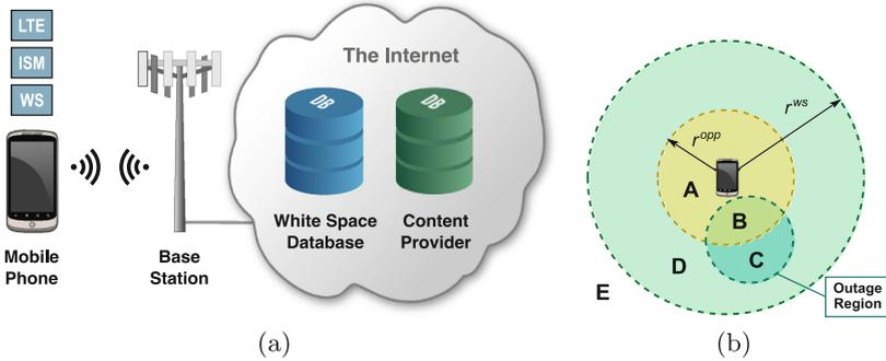
**Fig. 1.** (a) Reference architecture and (b) offloading regions: opportunistic offloading takes place in zones A and B, white space offloading in zone D, while no offloading is possible in zones C and E.
