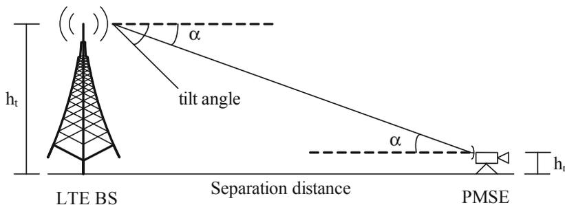
**Fig. 3.** Geometry between interfering transmitter and victim receiver.
