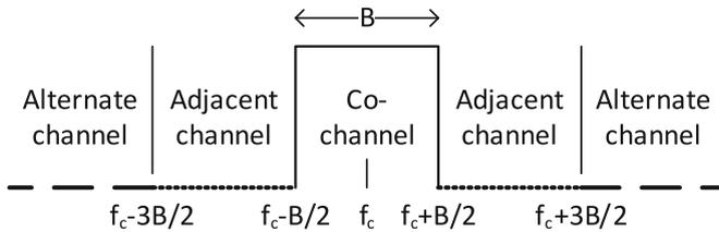
Fig. 2. Measurement mask normalized to channel bandwidth.
