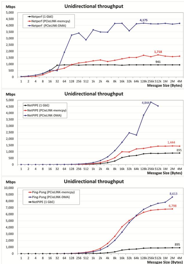
**Fig. 6.** The comparison of unidirectional throughput between Gigabit Ethernet (i.e. 1 GbE in the legend) and the proposed PCIeLINK. PCIeLINK-memcpy represents the results obtained with the memcpy data moving mechanism and PCIeLINK-DMA denotes the results obtained with the DMA data moving mechanism in the device driver. Peak values are noted in the figure.
