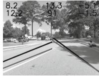
Fig. 5. False positive trusted line due to shadow condition.
