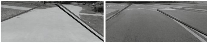
Fig. 6. Successful lane boundary detection on curved roads.
