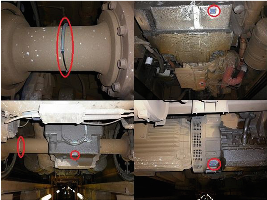
Fig. 1. Example of using RFID technology with integrated sensors for rail freight carriage.
