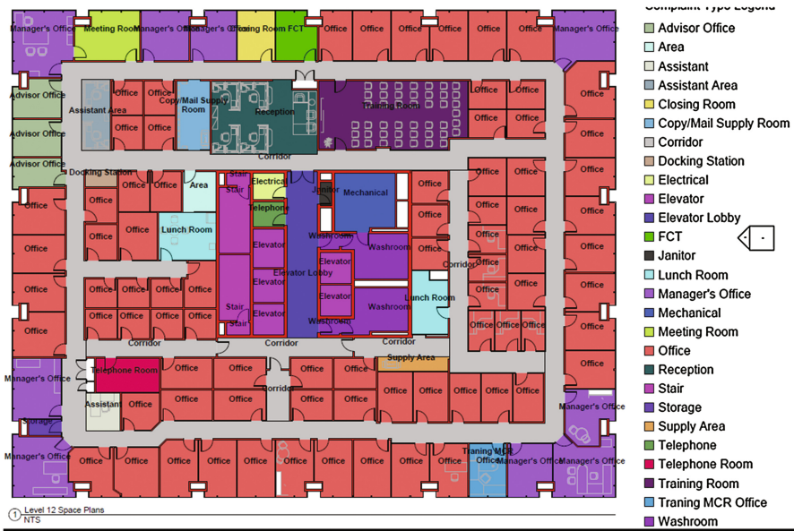
Fig. 6. Sample space management output from BIM model. (Color figure online)
