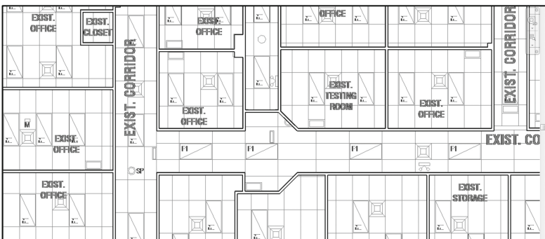
Fig. 2. Partial reflected ceiling plan of Facility A showing base geometry with overlaid 2D CAD data shown in grey.
