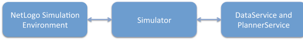
Fig. 1. Conceptual architecture of the simulation toolbox. The NetLogo multi-agent simulation environment is used as engine driving the simulation. The DataService and PlannerService are utility components providing information about the underlying transportation network and planning multi-model journeys, respectively.
