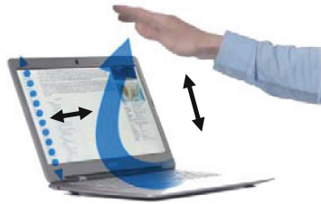
Fig. 1. An illustration of hand gesture recognition via sound waves used to control applications on laptop.
