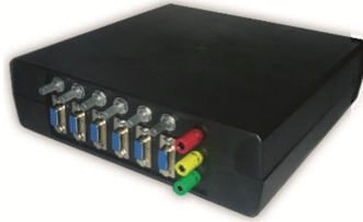
Fig. 5. Multichannel photoplethysmography device with six channels for PPG sensors, potentiometers for adjusting of PPG wave and three connectors for ECG electrodes.
